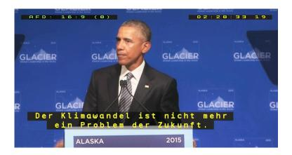
The inserter provides the option for graphical overlay. So any information like subtitles, AFD-status or timecode can be displayed on top of the videosignal for monitoring and control.
